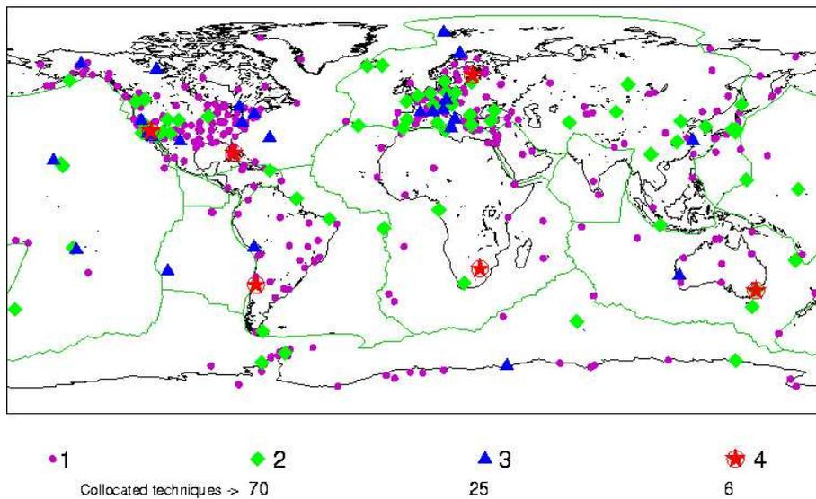
Figure 7: Global network of sites used in the determination of ITRF2000.
